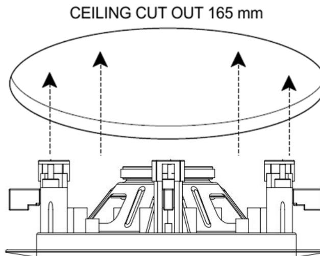
Once the hole is cut, remove the protective metal grille and insert the speaker in the hole.
